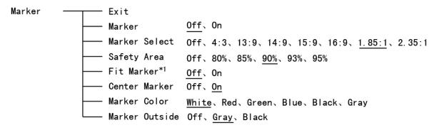
\*1 When "Fit Marker" is Off, the size of safety area is benchmarked against the actual display screen, accounting for  $80\% \sim 95\%$  of actual display screen. When "Fit Marker" is On, the size of safety area is benchmarked against the area inside the scales marker, accounting for  $80\% \sim 95\%$  of the area inside the scales marker.
