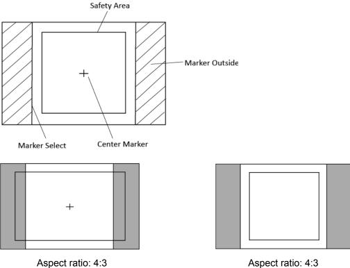
Aspect ratio: 4:3 Safety Area: 85% Center Marker: On Fit Marker: Off
